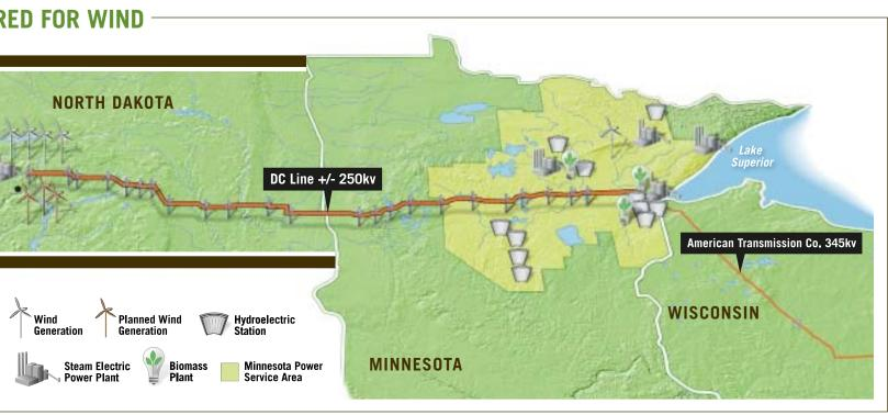
PICTURED LEFT: A 465-mile transmission line traversing northern forests will carry renewable wind energy to a Minnesota Power substation.
