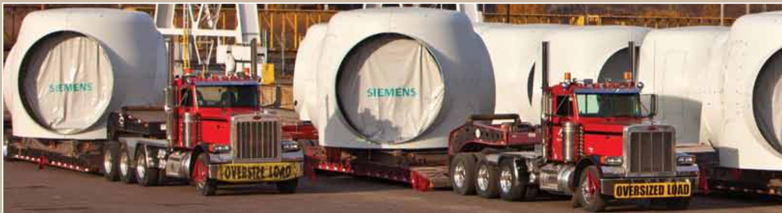
Hub assemblies for the Bison 1B wind farm are loaded onto trucks in Duluth, Minn. in early November for transport to North Dakota.
